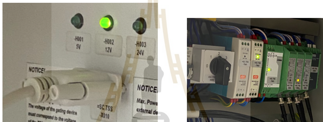
(a) The DB9 female sub connector of TSS interface box. (b) The inside of TSS interface box.
