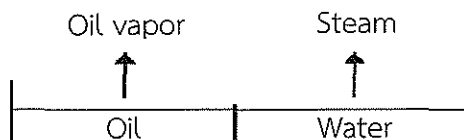
Figure 6.4 Each component of an immiscible liquid mixture contributes to the total vapor pressure as if the other component were not present
