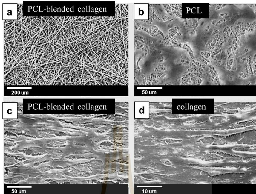
**Figure 2.4** SEM images of HDF cultured for 6 days on electrospun nanofibers. (a) PCL-blended collagen nanofibers, (b) HDF on PCL nanofibers, (c) HDF on PCL-blended collagen nanofibers, (d) HDF on collagen nanofibers. Modified from (Venugopal et al., 2007).
