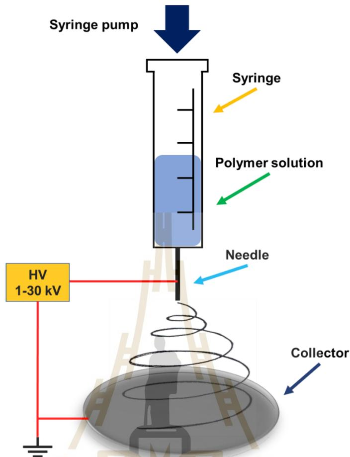
**Figure 2.1** Schematic of electrospinning setup.
