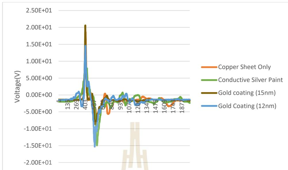
**Figure 4.26** Open voltage response as a function of electrode attachment to the piezoelectric fibers.
