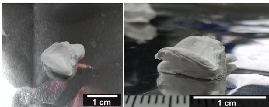
**Figure 4.3** The PVDF-HFP fibers after dried at room temperature (distance between needle and collector of 5 cm).
