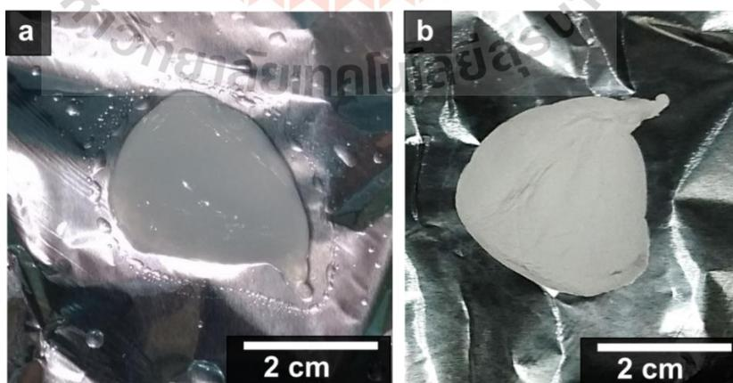
**Figure 4.4** The PVDF-HFP fibers (a.) after electrospinning and (b.) dried in room temperature (distance between needle and collector of 10 cm).
