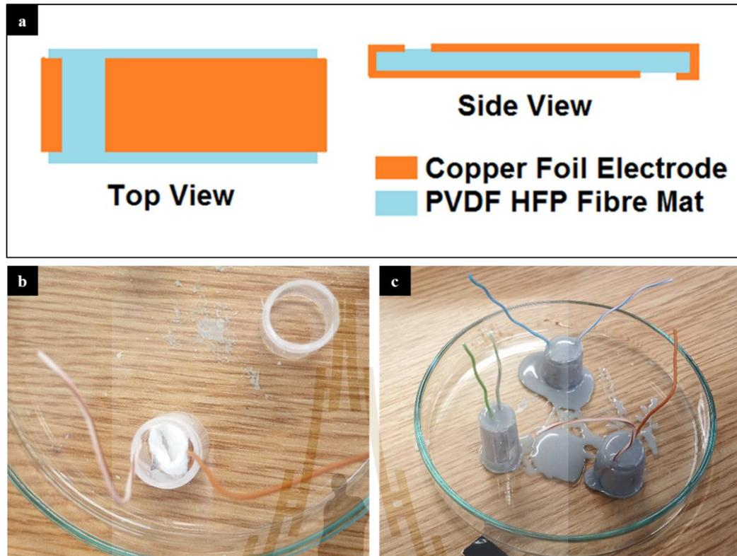
**Figure 4.23** Preparation of the 3D PVDF-HFP fibers sample for piezoelectric testing.
