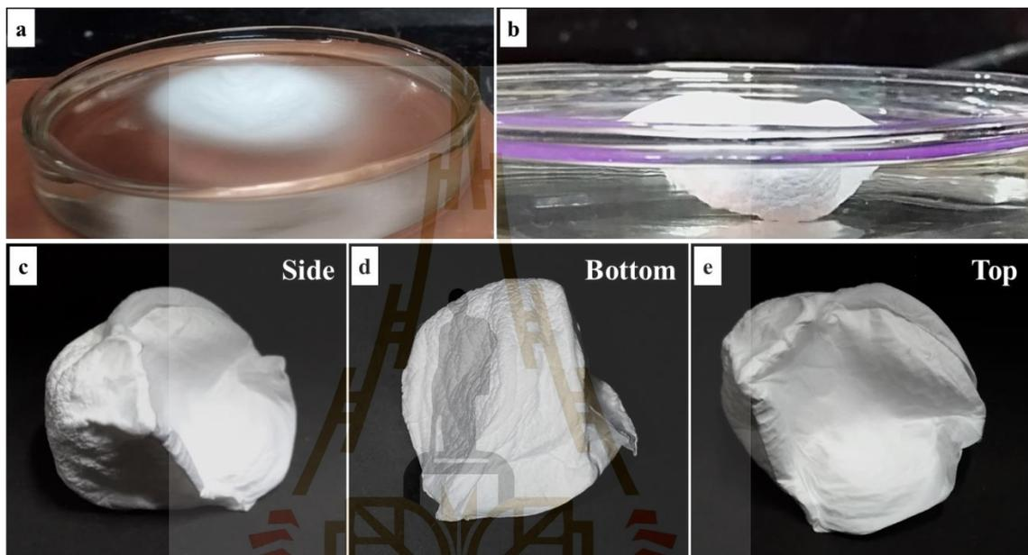
**Figure 4.6** The PVDF-HFP fibers (a) floated on the water and slightly collapsed, (b) were pulled down into the water by the weight of stacking fibers, (c), (d) and (e) show the 3D nanofibers scaffold from each side.
