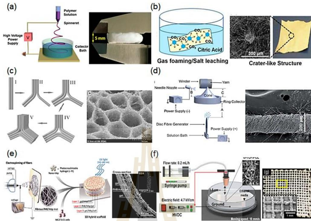
**Figure 2.12** 3D fibrous scaffolds using different electrospinning process: (a) liquid-collecting electrospinning; (b) gas foaming; (c) self-assembly; and (d) fibrous yarn scaffolds; (e) schematic illustration of a hydrogel-integrated fibrous scaffold; (f) a hybrid system using 3D printing and electrospinning. (Jun et al., 2018).
