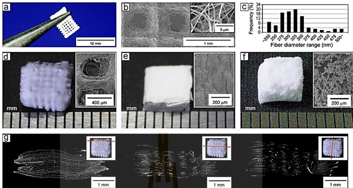
**Figure 2.10** Characterization of a patterned nanofibrous mat: (a) photograph, (b) SEM images, and (c) nanofiber diameter distribution. Photographs of 3D scaffolds fabricated using (d) the proposed method, (e) conventional electrospinning, and (f) salt leaching. (g) Micro-CT images of the scaffold shown in (d). (Lee et al., 2012).
