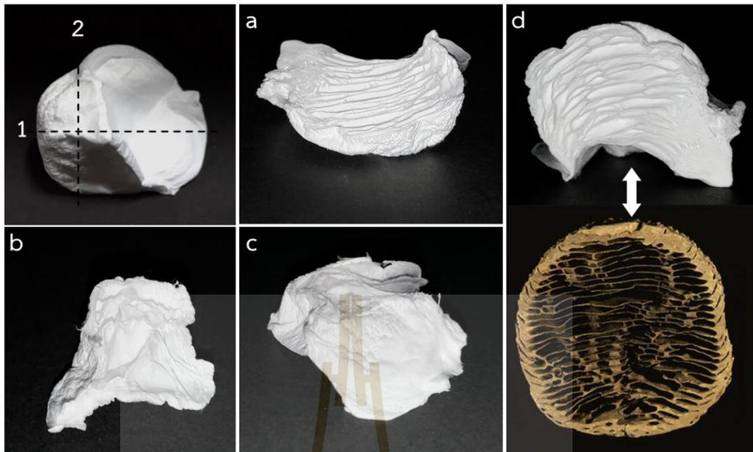
**Figure 4.13** Cross-section of 3D nanofibers scaffold cut through (a) line number 1, (b) and (c) line number 2, (d) compared with a termite (*Apicotermes*) nest. (Mermet G., 2019 from <http://www.savoirs.essonne.fr>).
