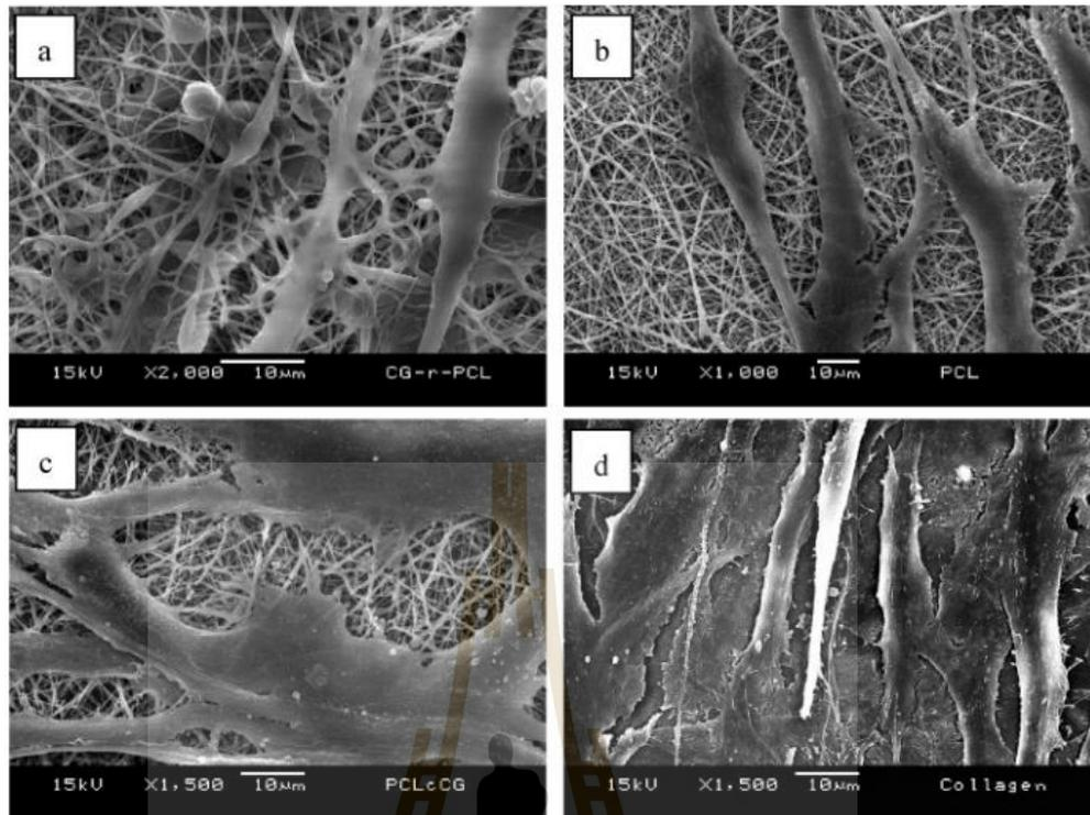
**Figure 2.8** A comparison of cells ingrowth behavior on different nanofibrous scaffolds: (a) core-shell collagen-PCL (Col-r-PCL); (b) pure PCL; (c) PCL with surface roughly collagen coated; and (d) pure collagen nanofibers. (Zhang et al., 2005).
