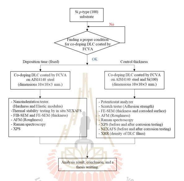
**Figure 3.1** The procedure chart of project activities for research on the topic of nanomechanical properties, thermal stability, and corrosion resistance of aluminium and nitrogen doped diamond–like carbon film
