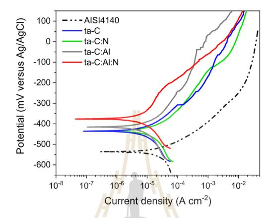
Figure 4.16 The polarization curves of AISI 4140, ta–C, ta–C:N, ta–C:Al, and ta–C:Al:N in 3.5 wt% NaCl solution, respectively (Wongpanya *et al.*, 2022)
