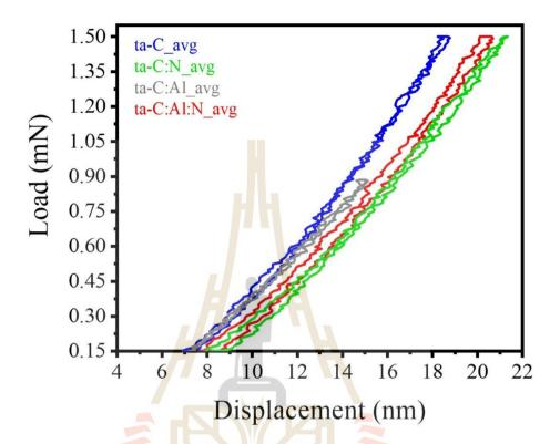
Figure 4.11 Load-displacement curves of ta-C, ta-C:N, ta-C:Al, and ta-C:Al:N (Wongpanya, Silawong, & Photongkam, 2021)
