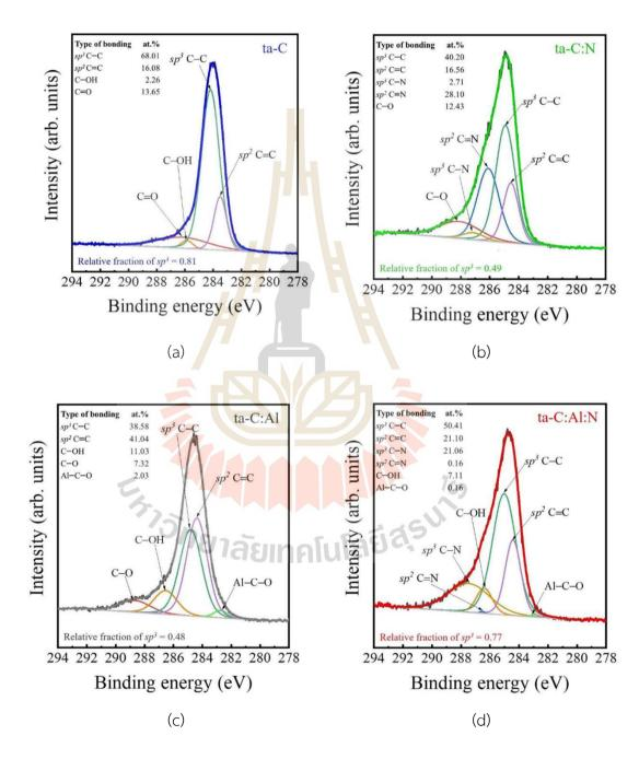
**Figure 4.2** The C 1s XPS spectra and corresponding deconvoluted Gaussian peaks of (a) ta–C, (b) ta–C:N, (c) ta–C:Al, and (d) ta–C:Al:N. (Wongpanya, Silawong, & Photongkam, 2021)
