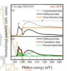
Fig. 9. In-situ high-temperature NEXAPS C.K.-edge spectrum generated for ta-C: AEN (a) price to data subtraction (where error function step was applied to fit edge jumping at inmination posential, as indicated in orange) and (b) after data subtraction (where spectrum was deconvoluted into multiple Gaussian peaks).
