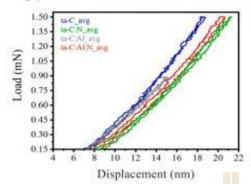
Fig. 5. Load-displacement curves of ta-C, ta-CN, ta-CAL and ta-CALN
