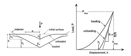
Figure 2.8 Schematic of the load and displacement curve, and deformation surface (Oliver and Pharr, 2004)
