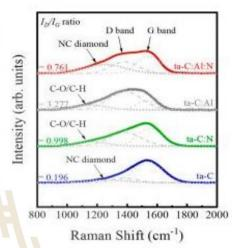
Fig. 2. Remon spectra of ta-C, ta-CN, ta-CAL and ta-CAEN.
