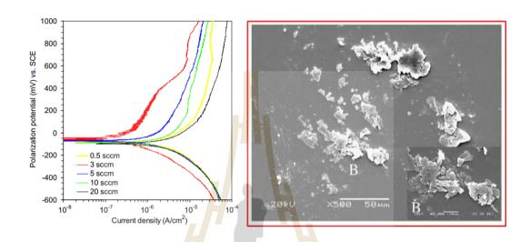
Figure 2.13 The polarization curve of ta–C:N and SEM image after potentiodynamic polarization test (Khun *et al.*, 2009).
