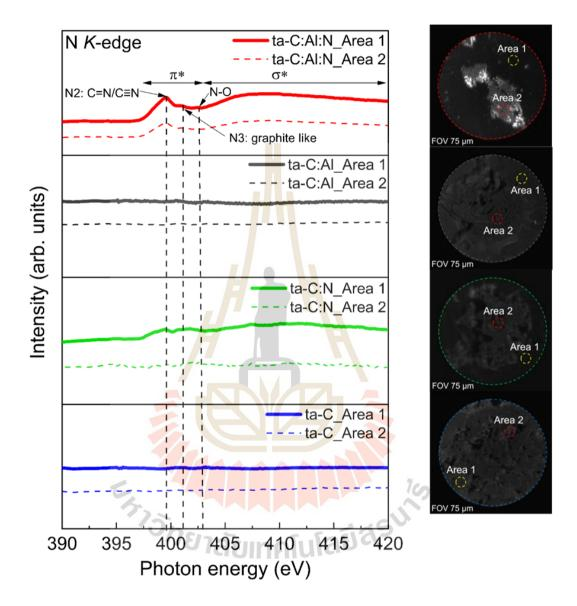
**Figure 4.19** The N K-edge NEXAFS spectra generated for ta-C, ta-C:N, ta-C:Al, and ta-C:Al:N after the corrosion tests (Wongpanya *et al.*, 2022)
