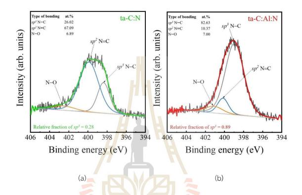
Figure 4.3 The N 1s XPS spectra and corresponding deconvoluted Gaussian peaks of (a) ta–C:N, and (b) ta–C:Al:N (Wongpanya, Silawong, & Photongkam, 2021)
