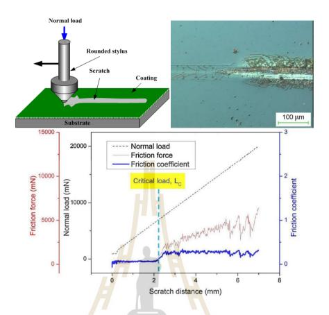
Figure 2.9 The schematic of a scratch tester, the result of the scratch test, and a microscope image of the damaged features at the critical ( $L_c$ ) (Bootkul et al., 2014; Tay et al., 2000)
