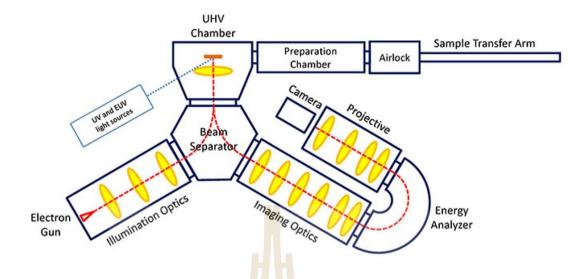
Figure 2.10 chematic of spectroscopic photoemission and low electron microscope (SPELEEM) [Online], Available: https://groups.oist.jp/fsu/leem-peem
