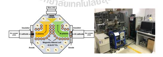
**Figure 3.2** Schematic of developed FCVA technique for synthesis films (Wongpanya *et al.*, 2022)
