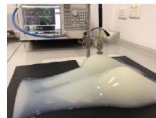
Fig. 4. Measurement setup for dielectric properties.
