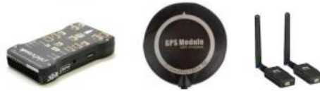
Figure 4(left): Pixhawk PX4 Figure 5 (center): GPS Module Figure 6 (right): 433Mhz Telemetry Set
