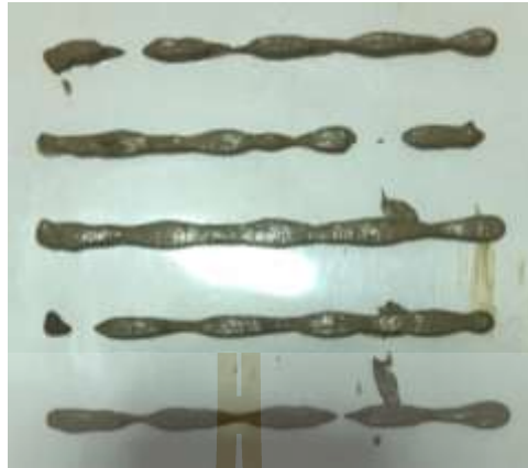
(a) Line test of extruded clay filament with formulation 1 (1:0:1)
