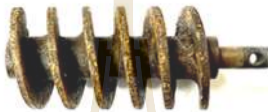
(b) the half pitch, single flight screw
