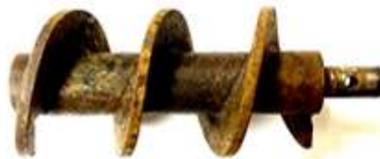
(a) the shot pitch, single flight screw
