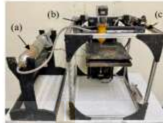
Fig. 3 The clay printing machine: (a) material container, (b) screw extruder, (c) movement system
