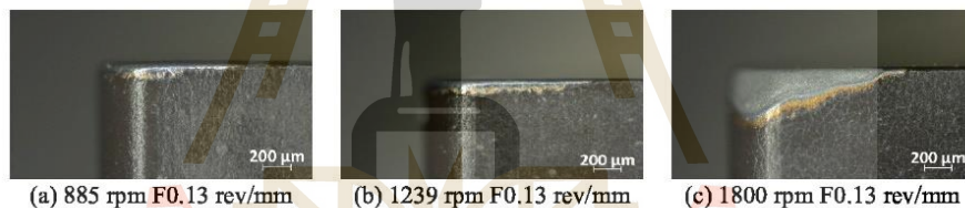
Figure 4. Tool wear under cryogenic.
