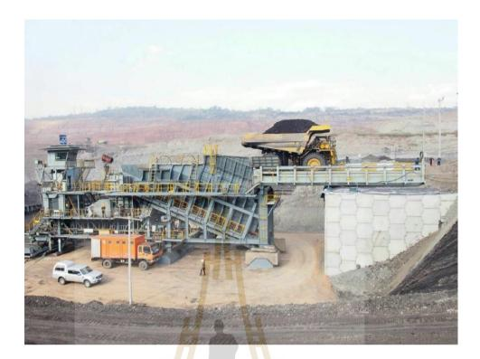
Figure 4.4 Photo of the BRE wall as a truck ramp support.
