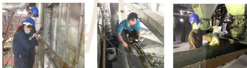
a) Surface temperature measurement b) Flue gas analysis c) Ash sample collection
