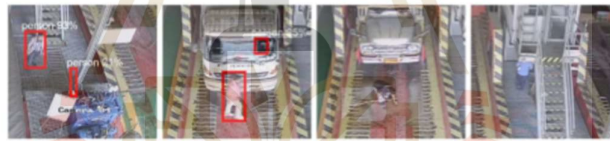
Figure 4. Example of false positive and false negative results from human detection system
