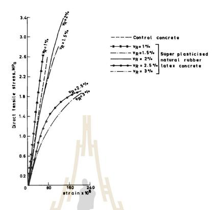
Figure 2.10 Stress-strain curves in tension of concrete with natural rubber latex (Nagaraj et al. 1988)
