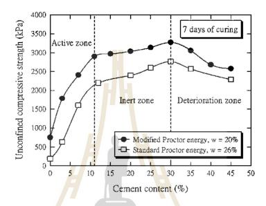
Figure 2.2 Strength developments as a function of cement content (Horpibulsuk et al. 2010)
