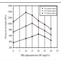
Fig. 6. Flexural strength at different cement contents and NRL replacement ratios.
