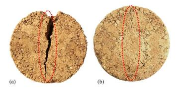
FIGURE 5.4 Failure characteristics of (a) cement stabilized soil A and (b) 20% NRL-cement stabilized soil A at C = 3% samples.
