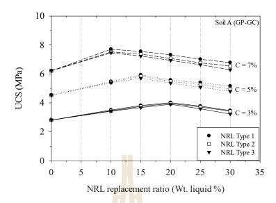
Figure 4.2 Unconfined compressive strength for different cement contents and NRL replacement ratios of NRL type 1, NRL type 2, and NRL Type 3 of Soil A.
