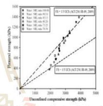
Fig. 7. Relationship between flexural strength and unconfined compressive strength
