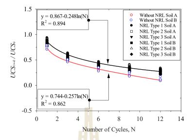
Figure 4.9 Relationship between UCS<sub>(w-d)</sub>/UCS<sub>0</sub> and number of w-d cycles at different cement contents and types of NRL for 0% NRL, 10% NRL, 15% NRL, 20% NRL, 25% NRL, and 30% NRL of Soil A and Soil B.
