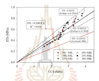
FIGURE 5.8 Relationship between ITS and UCS for cement stabilized Soil A, Soil B and Soil C with and without NRL at C = 3%, C = 5% and C = 7% for different NRL replacement ratios.
