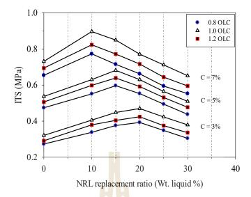
FIGURE 5.5 Indirect tensile strength for different cement contents and NRL replacement ratios of soil B at 0.8 OLC, 1.0 OLC and 1.2 OLC.
