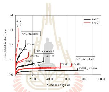
FIGURE 5.11 Relationship between number of cycles and horizontal deformation of cement stabilized Soil A and Soil C for C=3%, 0% and 20% NRL replacement ratios at 30%, 50%, and 70% stress level.
