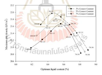
**Figure 3.2** The relationship between maximum dry density and optimum liquid content.
