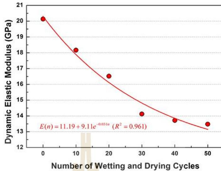
**Figure 2.2** Dynamic elastic modulus of specimens at the strain rate of  $90\text{s}^{-1}$  versus number of wetting and drying cycles (Zhou et al., 2017).
