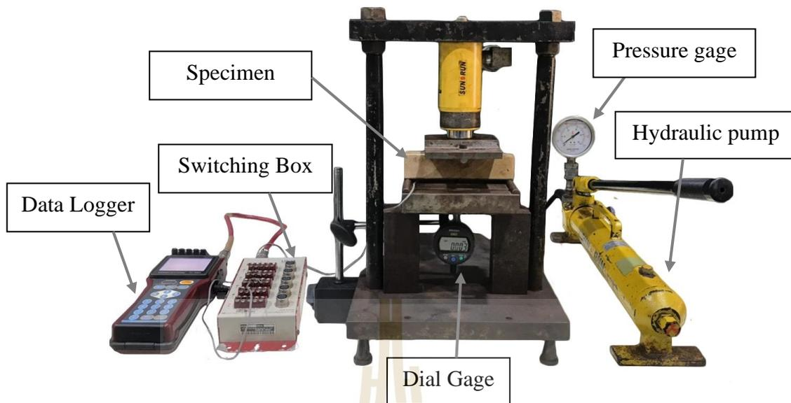
**Figure 4.3** Three-point bending test apparatus.
