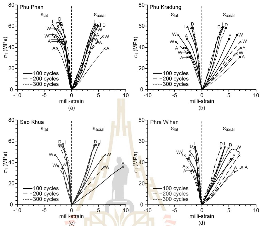
**Figure 5.7** Stress-strain curve from uniaxial compression tests for Phu Phan (a), Phu Kradung (b), Sao Khua (c), and Phra Wihan (d) sandstones under initial (I), dry (D), wet (W), and acid (A) condition.
