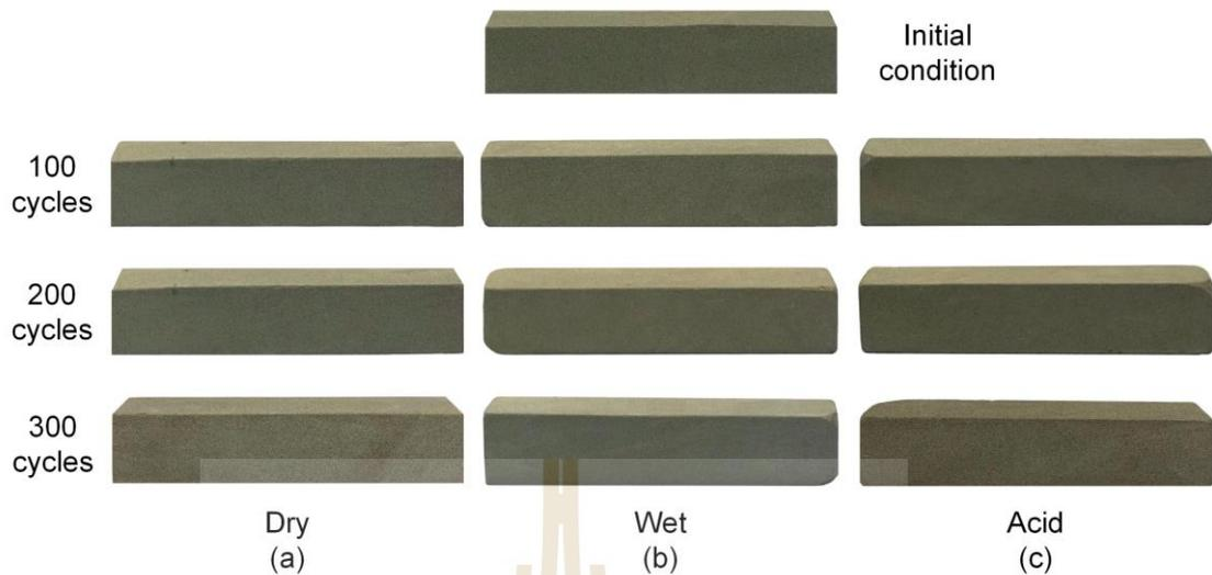
**Figure 5.2** Picture of Phu Kradung specimens through 100, 200 and 300 cycles under dry (a), wet (b) and acid (c) conditions.
