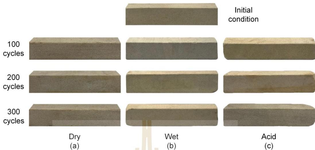
**Figure 5.4** Picture of Phra Wihan specimens through 100, 200 and 300 cycles under dry (a), wet (b) and acid (c) conditions.
