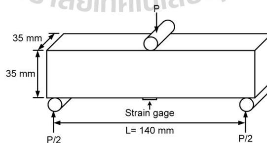
**Figure 4.2** Test arrangement for three-point bending test
