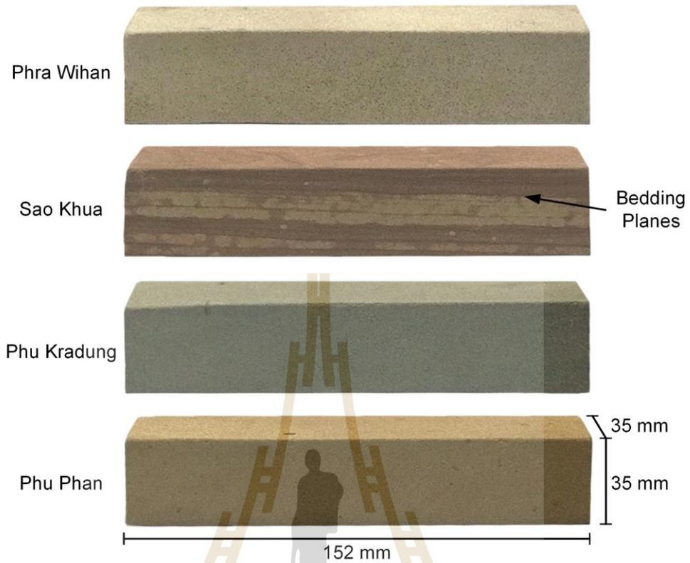
**Figure 3.1** Sandstone specimens prepared for simulation of degradation.
