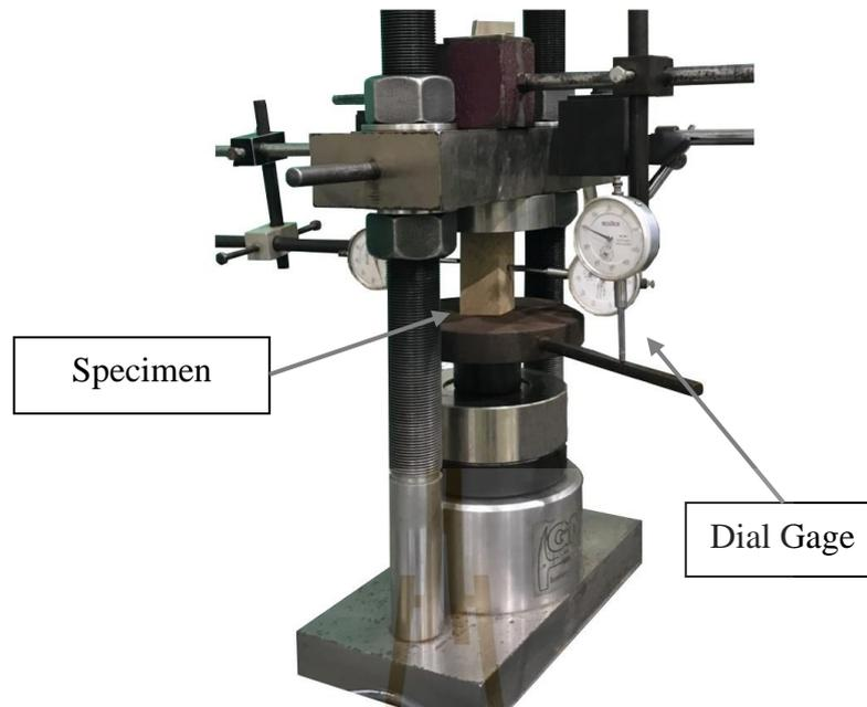
**Figure 4.4** Uniaxial compression test arrangement.
