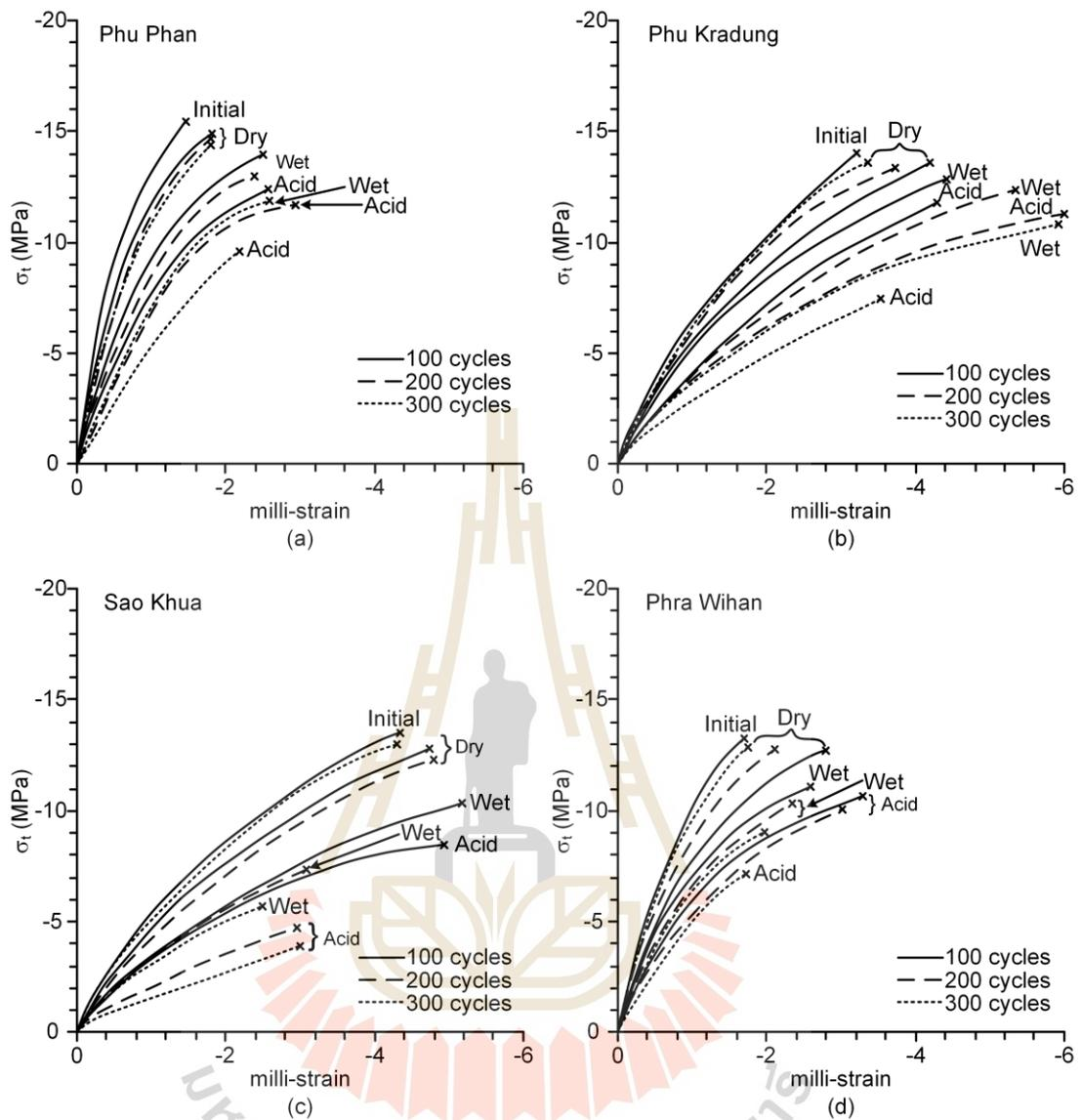
**Figure 5.8** Stress-strain curve from three-point bending tests for Phu Phan (a), Phu Kradung (b), Sao Khua (c), and Phra Wihan (d) sandstones.
