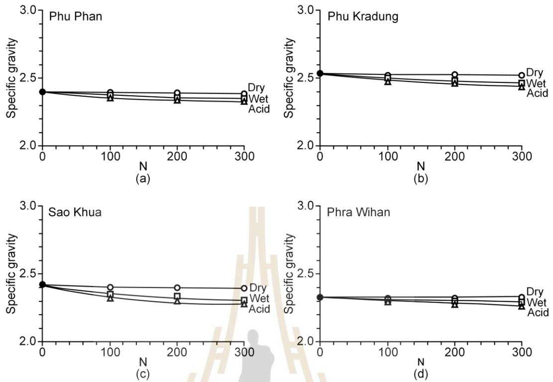
**Figure 6.1** The relationship curve between specific gravity and number of cycles (N) for Phu Phan (a), Phu Kradung (b), Sao Khua (c), and Phra Wihan (d) sandstones.
