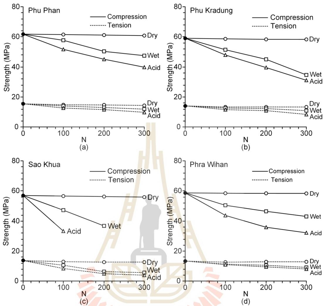
**Figure 5.6** Compressive and tensile strengths as a function of number of cycles (N) for Phu Phan (a), Phu Kradung (b), Sao Khua (c), and Phra Wihan (d) sandstones.
