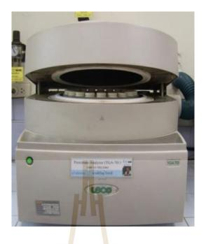
Figure 3.4 Leco TGA-701 (an automatic instrument for proximate analysis).
