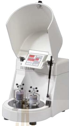
**Figure 2.10** Planetary ball mill machine (Fritsch Pulverisette-7)
