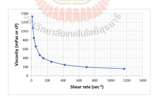
Figure 4.36 Relationship between shear rate and viscosity of SBL
