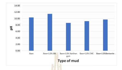
**Figure 4.34** The pH of drilling mud mixed with 1.0% of SBL, Xanthan gum, CMC, and Bentonite at 30°C.
