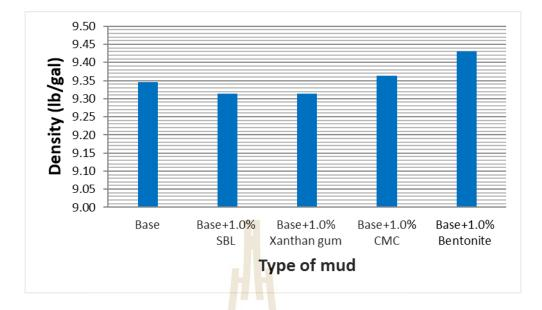
Figure 4.35 Density of drilling mud mixed with 1.0% of SBL, Xanthan gum, CMC, and Bentonite.
