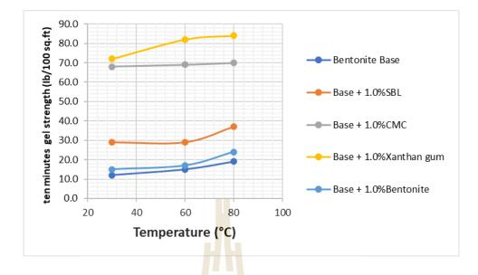
Figure 4.24 Ten minutes gel strength of drilling mud mixed with 1.0% of SBL, Xanthan gum, CMC, and Bentonite versus temperature.
