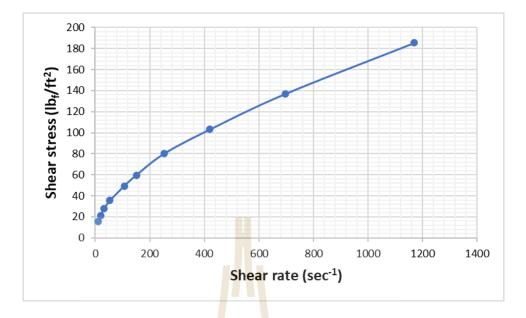
Figure 4.37 Relationship between shear rate and shear stress of SBL
