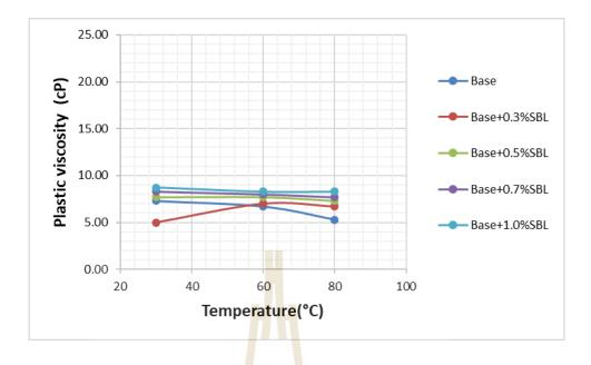
Figure 4.10 Plastic viscosity of drilling mud mixed with various SBL versus
