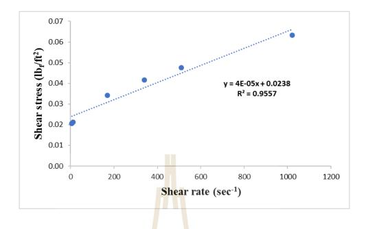
Figure 4.1 Consistency plot of base bentonite mud at 30°C with a linear correlation.
