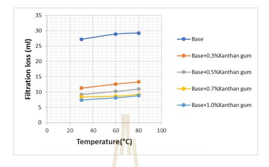
Figure 4.27 API filtrated loss of drilling mud mixed with Xanthan gum concentration
