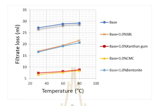
Figure 4.29 API filtrated loss of drilling mud mixed with 1.0% of SBL, Xanthan gum, CMC, and Bentonite versus temperature at 30 minutes.
