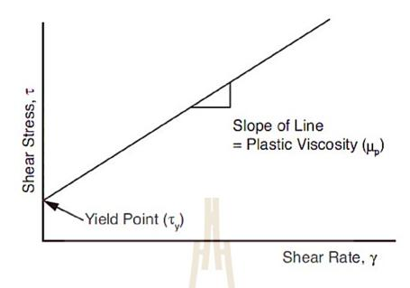
Figure 2.1 Flow curve for the Bingham plastic model
