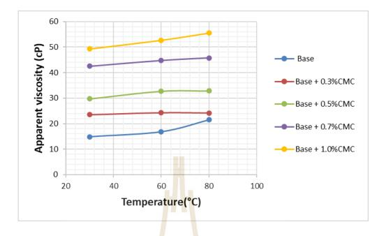
Figure 4.8 Apparent viscosity of drilling mud mixed with various CMC versus
