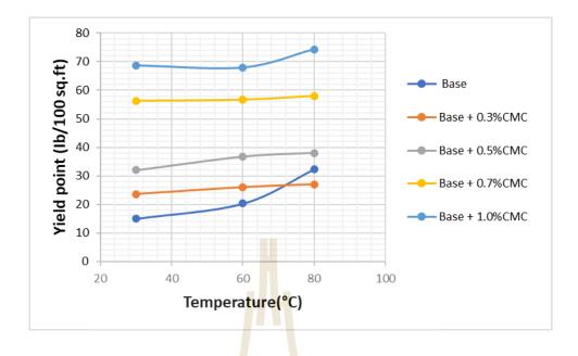
Figure 4.16 Yield point of drilling mud mixed with various CMC versus temperature.
