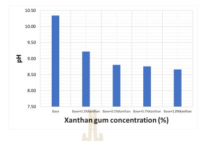
Figure 4.32 The pH of drilling mud mixed with various concentrations of Xanthan
