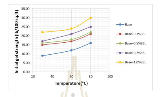
Figure 4.18 Initial gel strength of drilling mud mixed with various SBL versus
