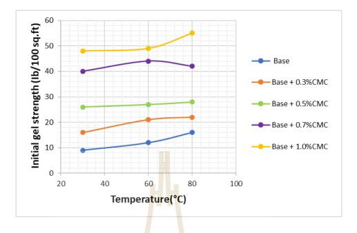
Figure 4.20 Initial gel strength of drilling mud mixed with various CMC versus
