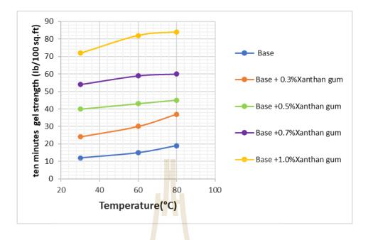
Figure 4.22 Ten minutes gel strength of drilling mud mixed with various Xanthan gum
