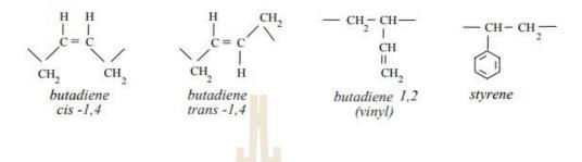
Figure 2.4 The general molecule structure of SBR (Matador, 2007)
