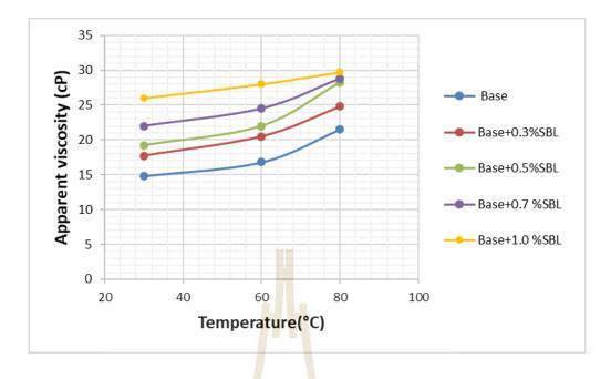
Figure 4.6 Apparent viscosity of drilling mud mixed with various SBL versus
