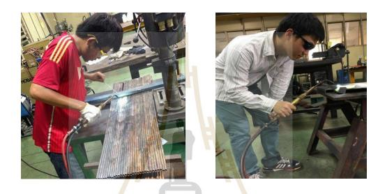
Figure 3.2 Welding copper tubes
