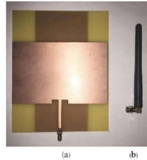
Fig.2 The proposed antenna used with NB-IoT module: (a) fabricated microstrip patch antenna (b) monopole antenna.
