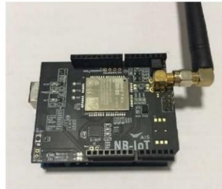
Fig 6 The DEVIO NB-SHIELD connected on Arduino Board.
