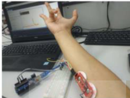
Fig. 6: photograph of an example of measurement using MyoWare Muscle Sensor.
