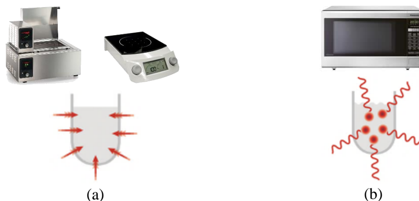
Figure 2.6 Schematic representation of heating : (a) Conventional heating and (b) Microwave heating
