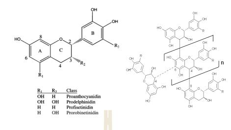
Figure 1 CT basial units and structure. source: Schofield et al., 2001.
