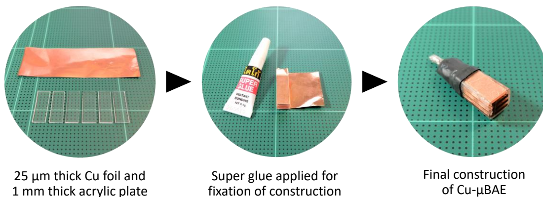
Figure 3.11 The making of copper microband array electrode with super glue as adhesive.
