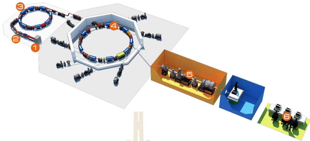
Figure 2.18 Schematic of synchrotron facility, (1) electron gun, (2) linear accelerator, (3) booster ring, (4) storage ring, (5) beamline, and (6) experimental station ( http:// www.slri.or.th ).
