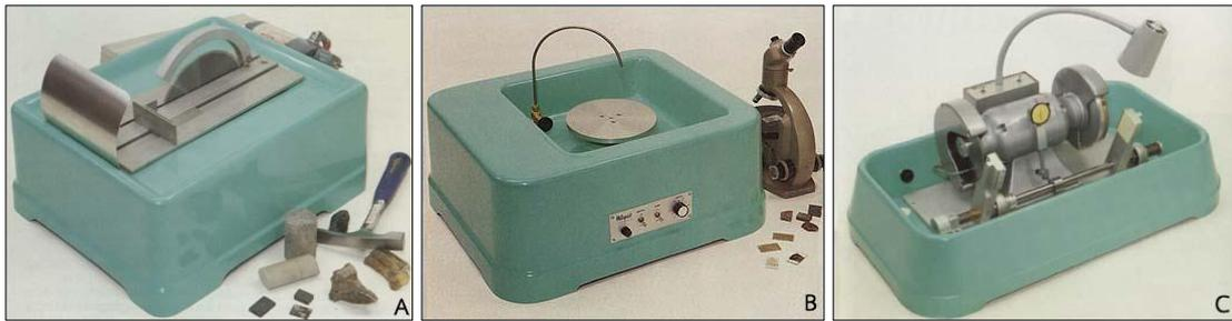
**Figure 3.3** The machine for the preparation of the polish slab and thin section. (A) The Hillquist SF-8 Trim saw machine (B) The Hillquist Thin Section Grinder machine (C) The Hillquist Thin Section machine (Seven republic, www, 2015).
