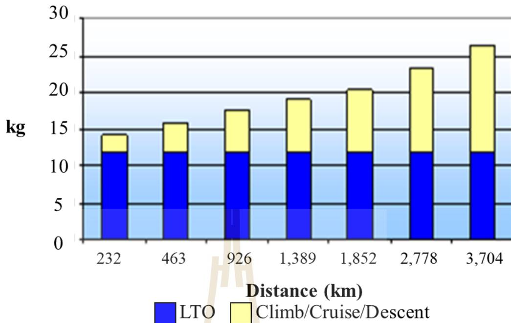
**Fig. 2.9** Carbon monoxide emission from the aircraft type B737 400
