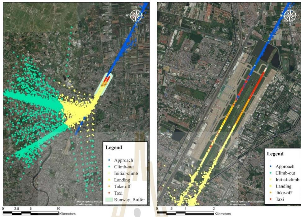
**Fig. D.2** The commercial aircraft movement at Don Mueang airport
