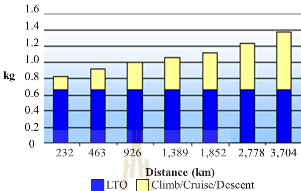
**Fig. 2.10** Hydrocarbon emission from the aircraft type B737 400
