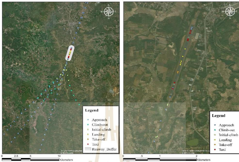
Fig. D.8 The commercial aircraft movement at Loei airport
