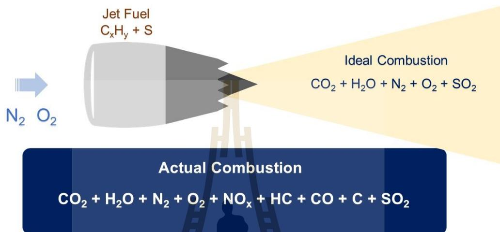
**Fig. 2.6** Emissions from combustion of aircraft's engine (Adopt from Weubbles et al. 2007; Norton, 2014)
