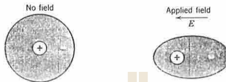
Fig. 13.8. Shift of electron cloud giving rise to dipole moment and electronic polarization.
