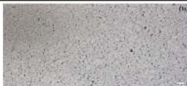
Fig.2. Microstructure of samples after solution treated (a) rolled Aluminium Alloy 2024 and (b) semi-solid casted aluminium alloy 2024
