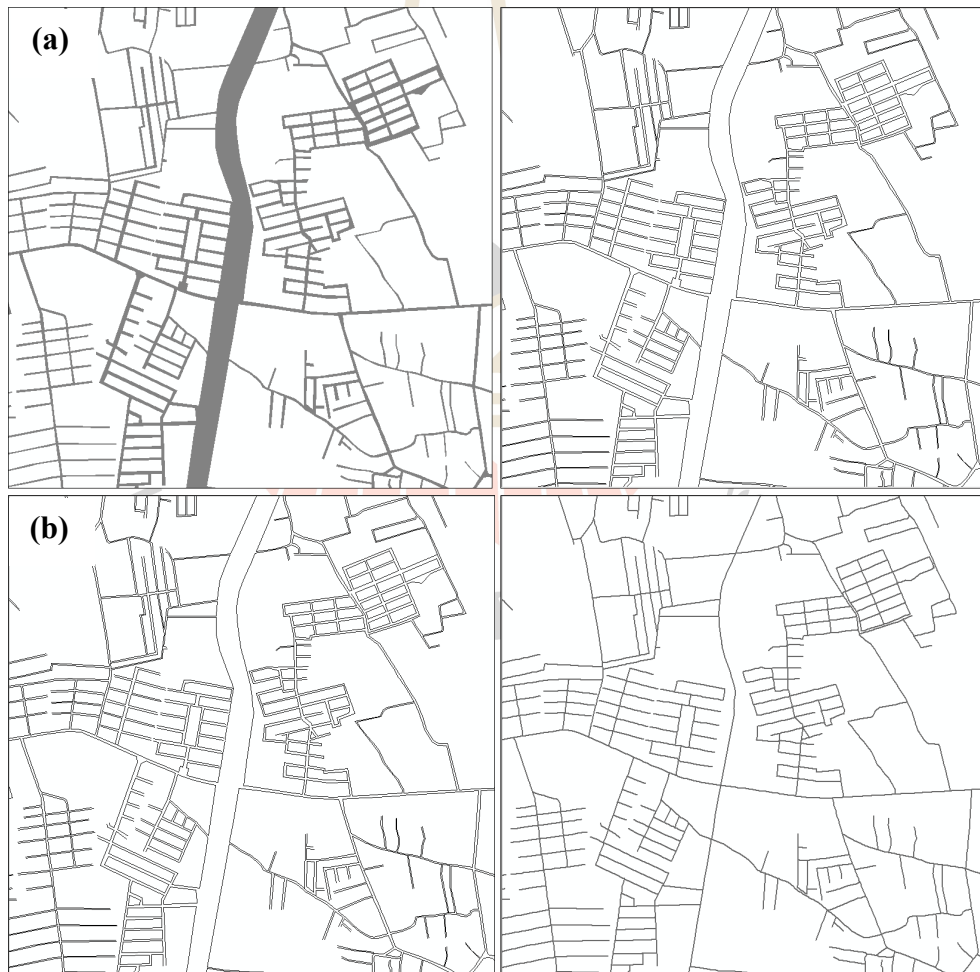
Figure 4.9 Road polygons from RS interpretation were converted to lines of polygon boundaries (a). Centerlines of road network were then generated from them (b).
