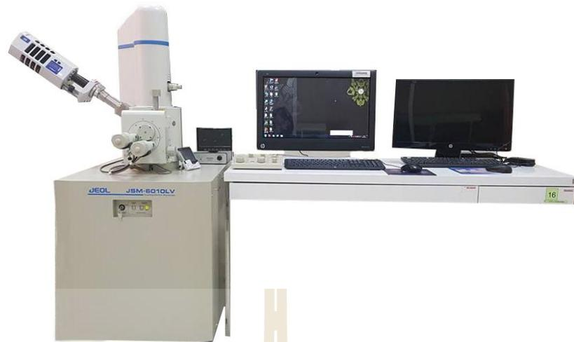
**Figure 6.1** JEOL JSM-6010LV scanning electron microscope used in this studied.
