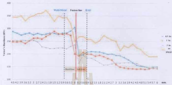
Fig. 4: Hardness profile across the weld interface before and after PWHT
