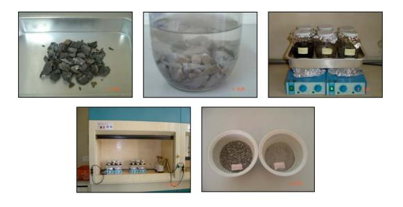
**Figure 3-2** Process of hot acetolysis performed at the Center of Scientific and Technological Equipment, Suranaree University of Technology.
