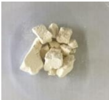
Figure 4.16 The photograph of pre-PLA product produced using condensation polymerization.
