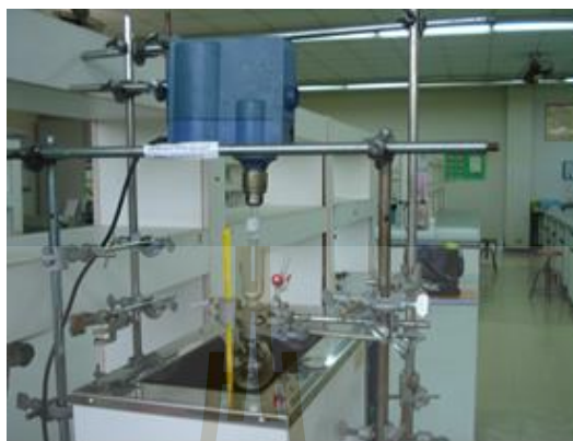
Figure 3.2 Photograph showing experimental set up for synthesis of PLA pre-polymer.
