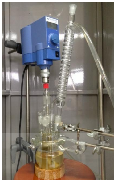
Figure 3.1 Photograph of a reactor setting for preparation of hydroxyl terminated natural rubber.
