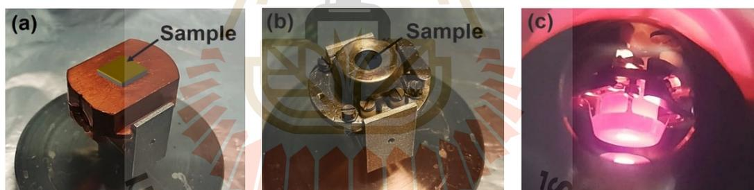
**Figure 3.15** Photographs of (a) the unheatable substrate holder, (b) heatable substrate holder, and (c) heatable substrate holder during annealing in X-PEEM main chamber.
