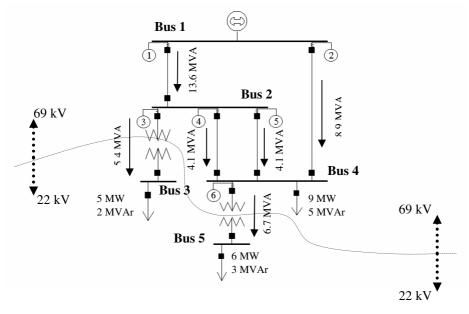
Fig. 1. Power flow solution for the maximum load operation
