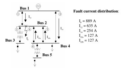
Fig. 2. Fault current distribution for the occurrence of fault at bus 2
