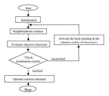
Fig. 6. Flow diagram for the ATS method
