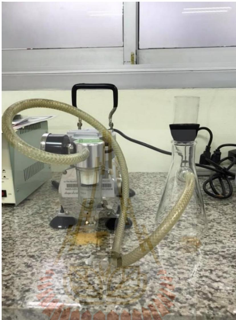
**Figure 3.6** The membrane synthesis via suction seeding method.
