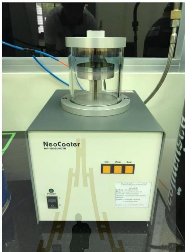
**Figure 3.9** Gold coating machine (Neo coater MP-19010 NCTR, JEOL, Japan).
