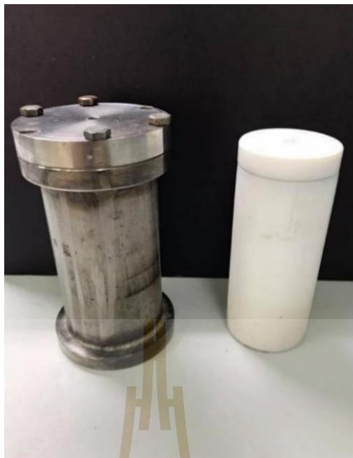
**Figure 3.4** 45 mL Teflon lined stainless steel autoclave.
