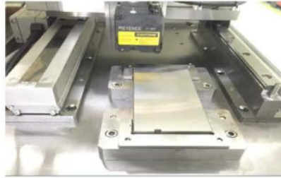
Fig 10 Calibration Master, size 10 mm
