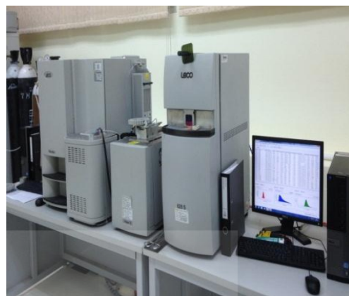
(h). C, H, N, S and O analyzer
