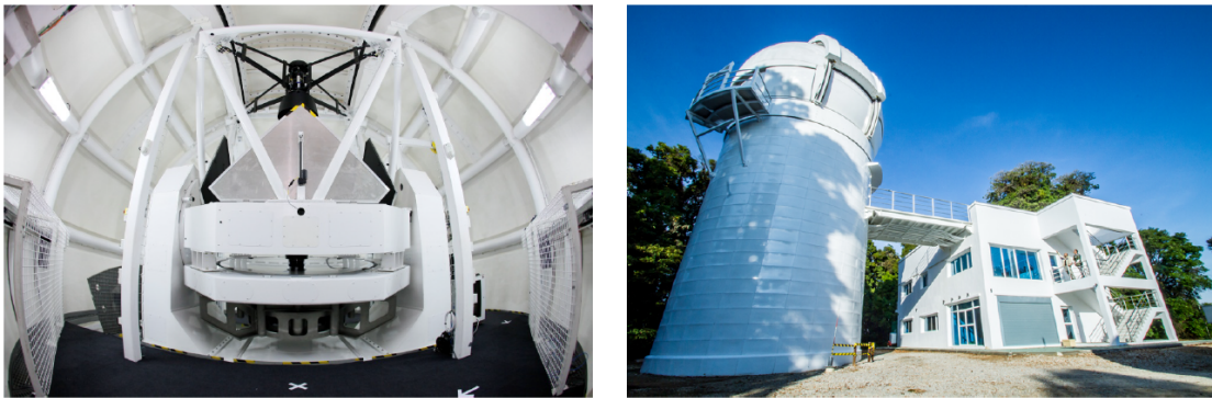
Figure B.2 Left: The mirror of Thai National Telescope (TNT) covers are open and the 2.4 m f/1.5 primary mirror can be seen towards the bottom. Right: Outside of the TNT is shown the tower on which the telescope sits and the adjacent control room building (Dhillon et al., 2014).
