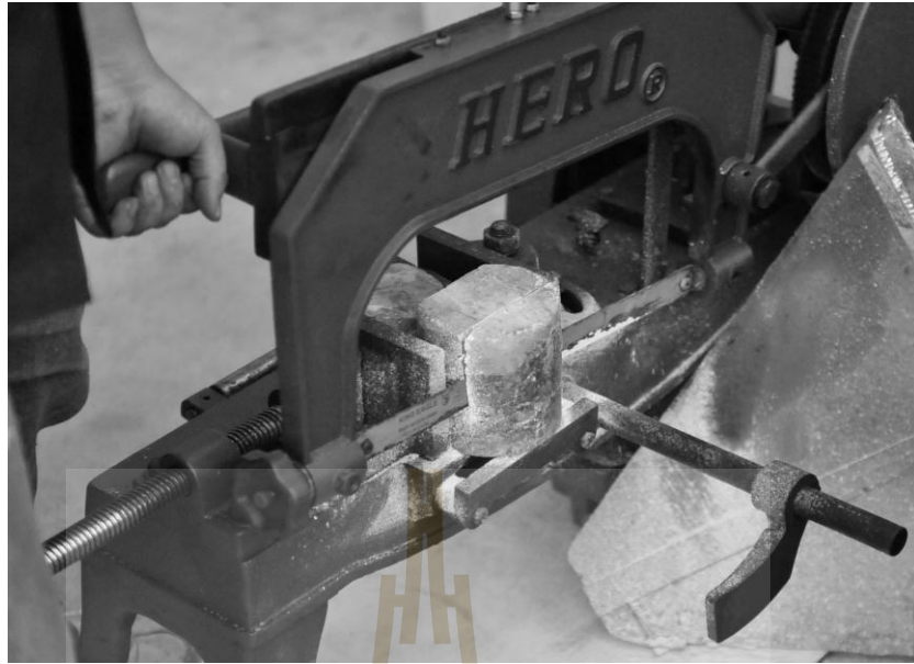
Figure 3.1 A salt specimen is dry cut by a cutting machine.
