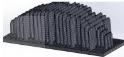
Fig. 3 Discretization of LED street lamp
