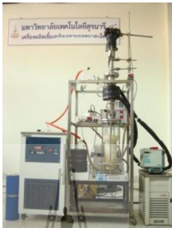
Figure 3.2 Experimental setup for extractive fermentation of ethanol using vacuum fractionation technique (A). Experimental set up in the laboratory (B).
