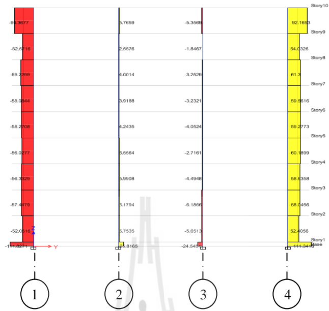
Figure 4.26 shows shear force diagrams in Elevation B.
