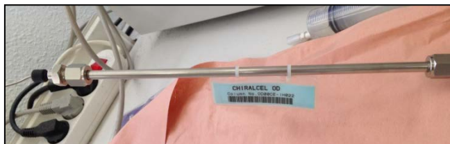
Figure B.10 Picture of a ChiralCel OD column used for analyzing the e.e.
