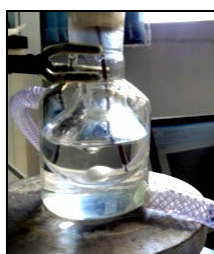
Figure B.2 Picture of the reactor used for the study of deracemization and preferential crystallization in the presence of racemization in solution.
