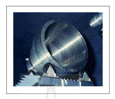
**Figure 2.5** The corrugated horn (Kay, 1962)
