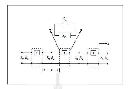
**Figure 3.9** The transmission line model of EBG structures (Rahman and Stuchly, 2001).
