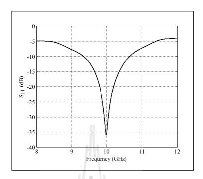
Figure 5.21 Simulated reflected power  $(S_{11})$  of a Type-D circular horn with PEC arm.
