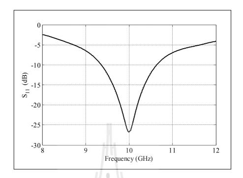
**Figure 5.6** Simulated reflected power  $(S_{11})$  of a Type-D rectangular horn with PEC arm.
