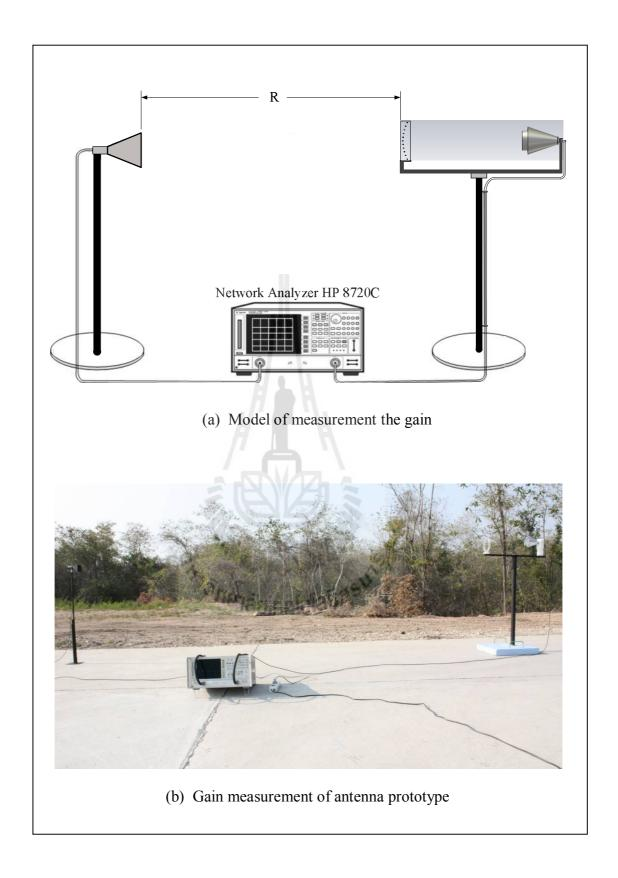
Figure 5.33 Gain measurement of the prototype of Type-D circular horn.
