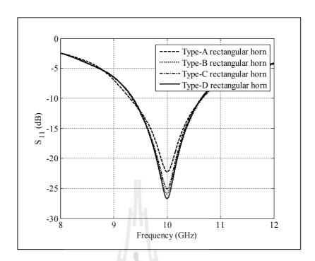
Figure 4.24 Simulated result of reflected power  $(S_{11})$  of four types of the rectangular horn antennas.
