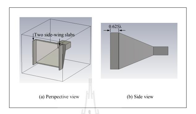
**Figure 4.16** A rectangular horn antenna with two side-wing slabs (Type-C rectangular horn).
