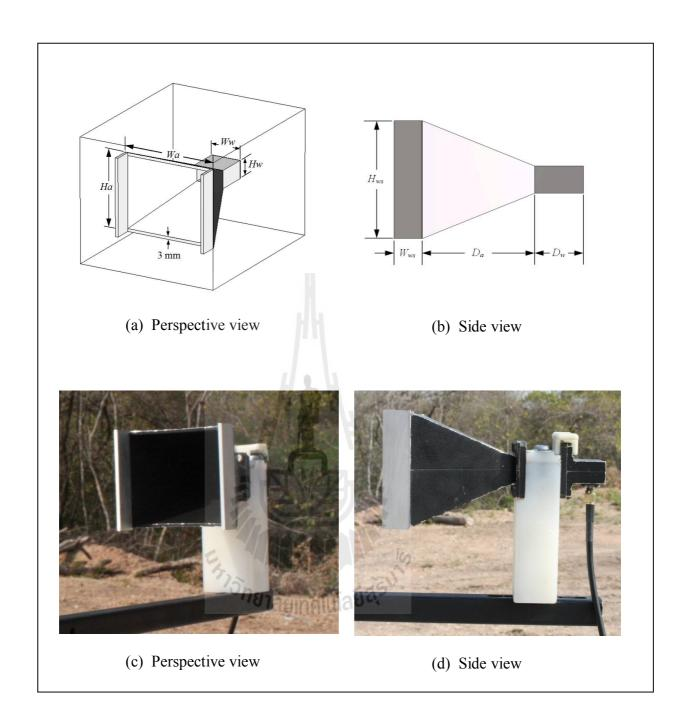
**Figure 5.2** Configuration and prototype of rectangular horn antenna with two side-wing slabs.
