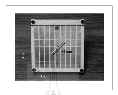
**Figure 2.9** A dipole antenna that radiates circularly polarized patterns (Yang and Rahmat-Samii, 2005).
