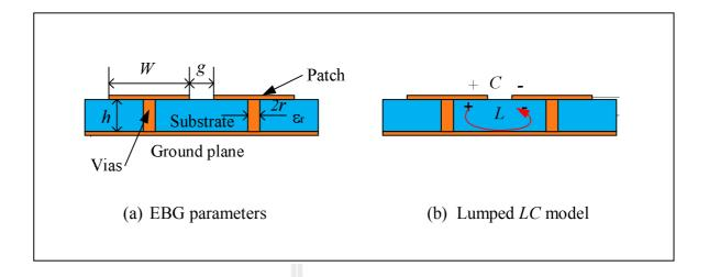
Figure 3.8 The lumped element model for the mushroom-like EBG structures.
