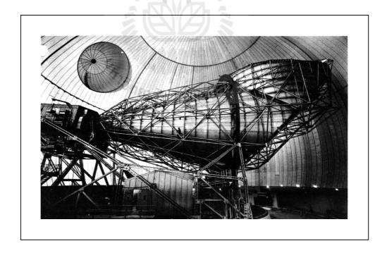
Figure 2.4 A large 177 ft. horn antenna (http://en.wikipedia.org).
