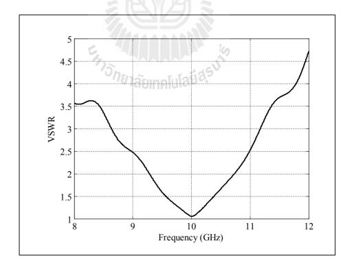
Figure 4.29 Simulated VSWR of a Type-A circular horn.
