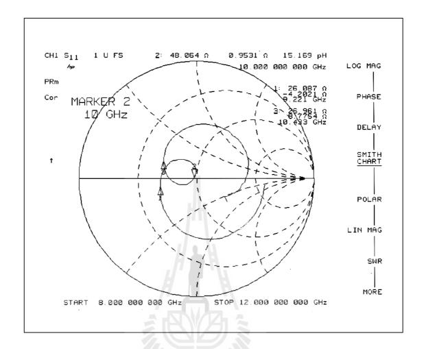
Figure 5.27 Measured input impedance of the prototype of Type-D circular horn.
