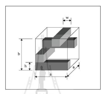
**Figure 3.11** A unit cell of four layers planar woodpile EBG structures (Weily *et al.*, 2005).
