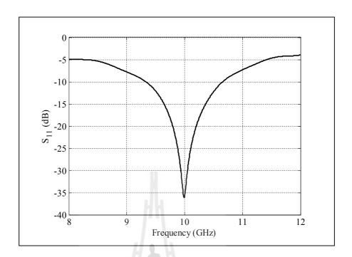
**Figure 4.32** Simulated result of reflected power  $(S_{11})$  of a Type-B circular horn.
