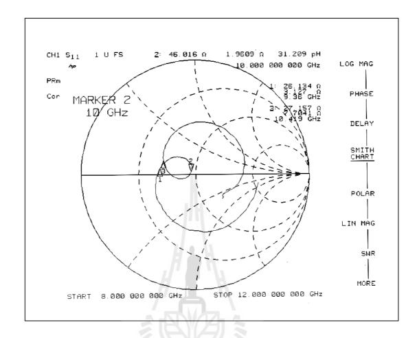
Figure 5.12 Measured input impedance of the prototype of Type-D rectangular horn.
