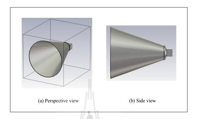
Figure 4.27 A conventional circular horn antenna and waveguide adapter (Type-A circular horn).
