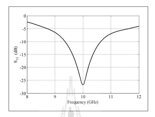
**Figure 4.21** Simulated result of reflected power  $(S_{11})$  of a Type-D rectangular horn.
