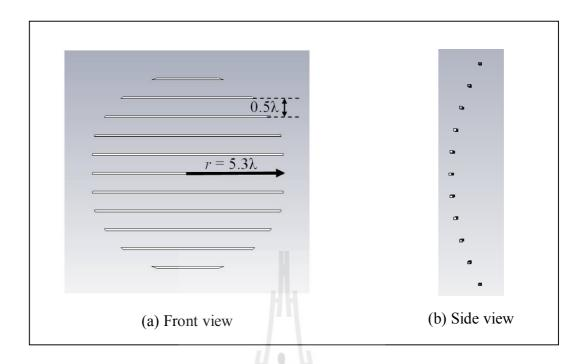
Figure 4.4 The configuration of quadratic shaped woodpile EBG structures.
