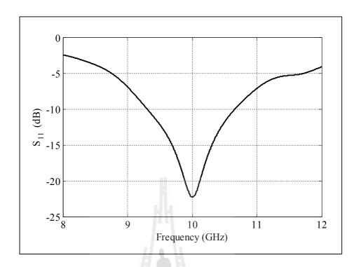
**Figure 4.9** Simulated result of reflected power  $(S_{11})$  of a Type-A rectangular horn.
