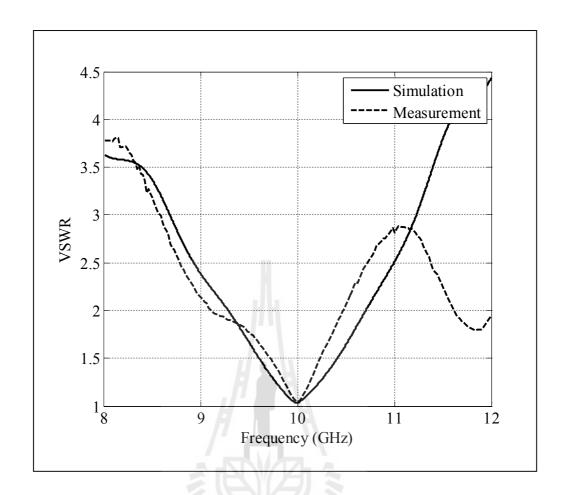
**Figure 5.29** Comparison between simulated and measured results of VSWR for the prototype of a Type-D circular horn.
