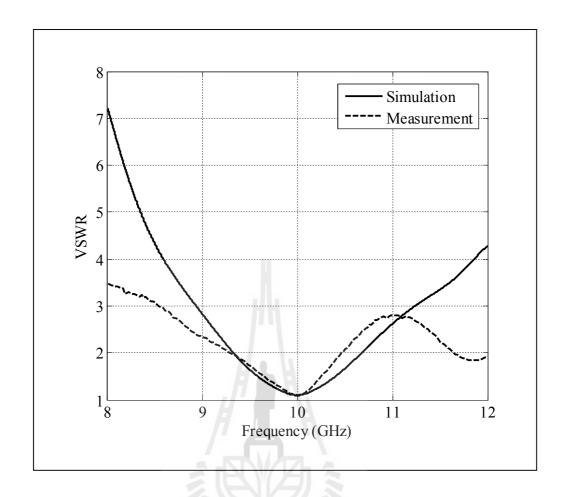
**Figure 5.14** Comparison between simulated and measured results of VSWR for the prototype of a Type-D rectangular horn.
