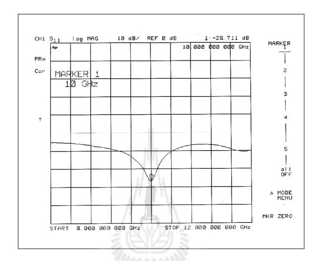
Figure 5.10 Measured reflected power  $(S_{11})$  of the prototype of a Type-D rectangular horn.
