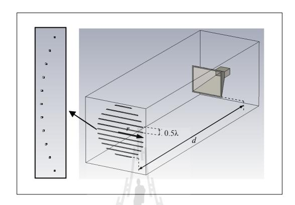
**Figure 4.12** A conventional rectangular horn antenna and the designed woodpile EBG (Type-B rectangular horn).
