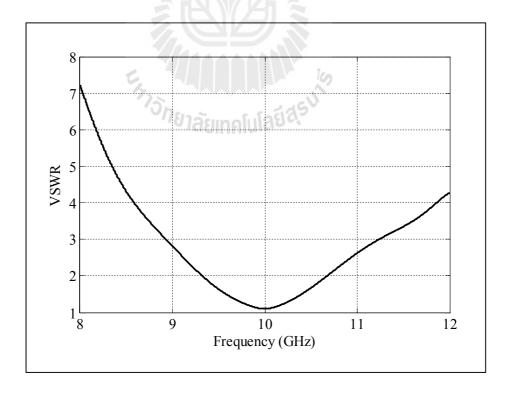
Figure 4.22 Simulated VSWR of a Type-D rectangular horn.
