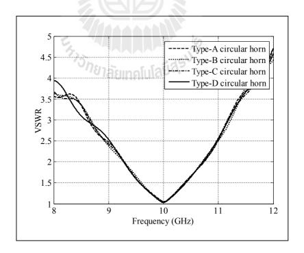
Figure 4.44 Simulated VSWR of four types of the circular horn antennas.
