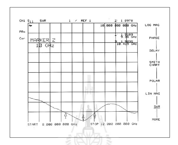
Figure 5.11 Measured VSWR of the prototype of a Type-D rectangular horn.
