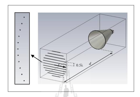
**Figure 4.31** A conventional circular horn antenna and the designed woodpile EBG (Type-B circular horn).
