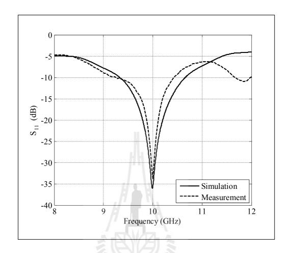
Figure 5.28 Comparison between simulated and measured results of reflected power  $(S_{11}) \ for \ the \ prototype \ of \ a \ Type-D \ circular \ horn.$
