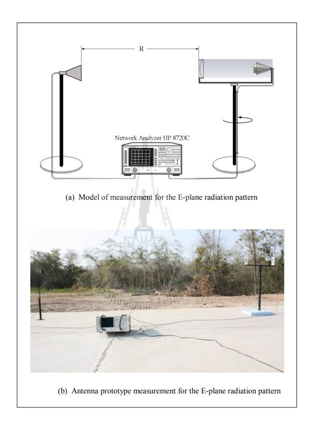
**Figure 5.31** Measurement set up for the radiation pattern of the prototype of Type-D circular horn.
