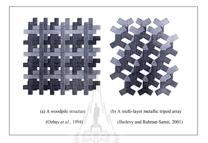
Figure 3.6 The 3D EBG volumetric structures.
