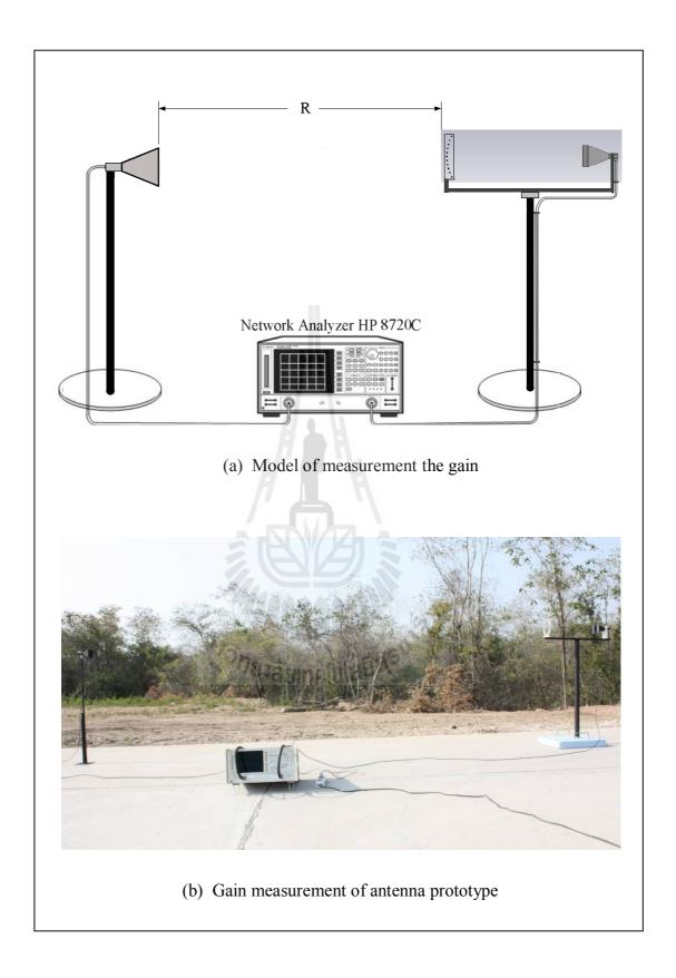
Figure 5.19 Gain measurement of the prototype of Type-D rectangular horn.
