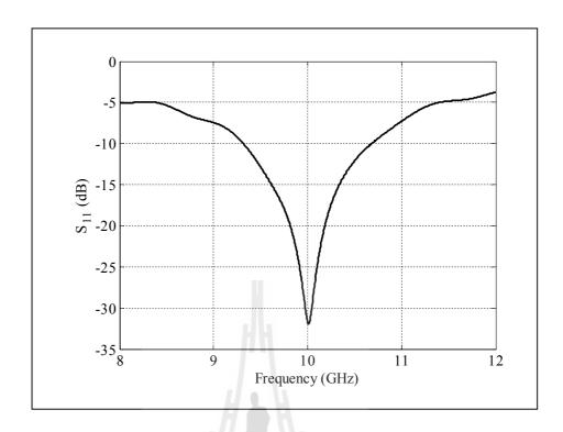
Figure 4.28 Simulated result of reflected power  $(S_{11})$  of a Type-A circular horn.
