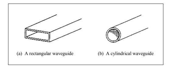
Figure 3.2 The geometry of the waveguides.
