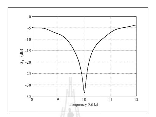
Figure 4.36 Simulated result of reflected power  $(S_{11})$  of a Type-C circular horn.
