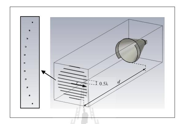
**Figure 4.39** A circular horn antenna with two side-wing slabs and the designed woodpile EBG (Type-D circular horn).
