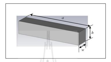
Figure 3.12 A unit cell of one layers planar woodpile EBG structures.
