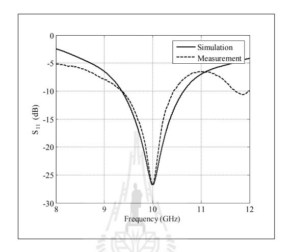
Figure 5.13 Comparison between simulated and measured results of reflected power  $(S_{11}) \ for \ the \ prototype \ of \ a \ Type-D \ rectangular \ horn.$
