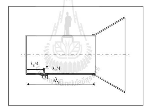
**Figure 3.3** A rectangular waveguide fed with a short monopole.
