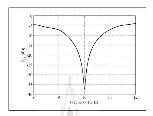
Figure 4.40 Simulated result of reflected power  $(S_{11})$  of a Type-D circular horn.
