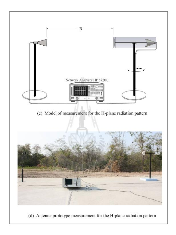
**Figure 5.31** Measurement set up for the radiation pattern of the prototype of Type-D circular horn (Continued).
