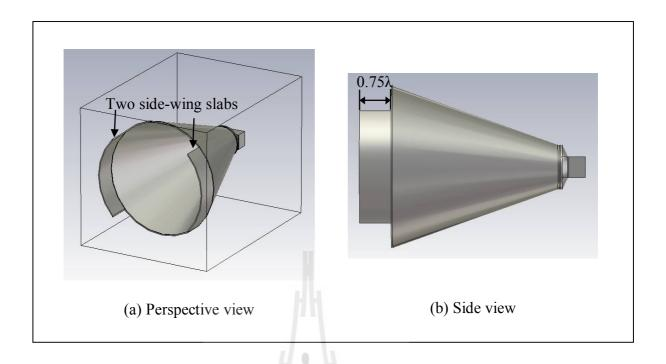
Figure 4.35 A circular horn antenna with two side-wing slabs (Type-C circular horn).
