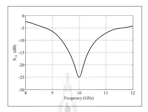
Figure 4.17 Simulated result of reflected power  $(S_{11})$  of a Type-C rectangular horn.
