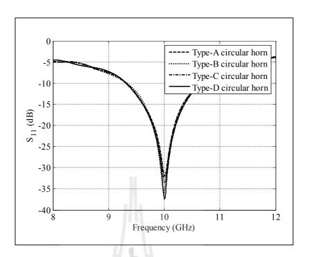
Figure 4.43 Simulated result of reflected power  $(S_{11})$  of four types of the circular horn antennas.
