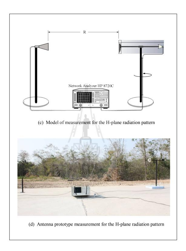
**Figure 5.16** Measurement set up for the radiation pattern of the prototype of Type-D rectangular horn (Continued).
