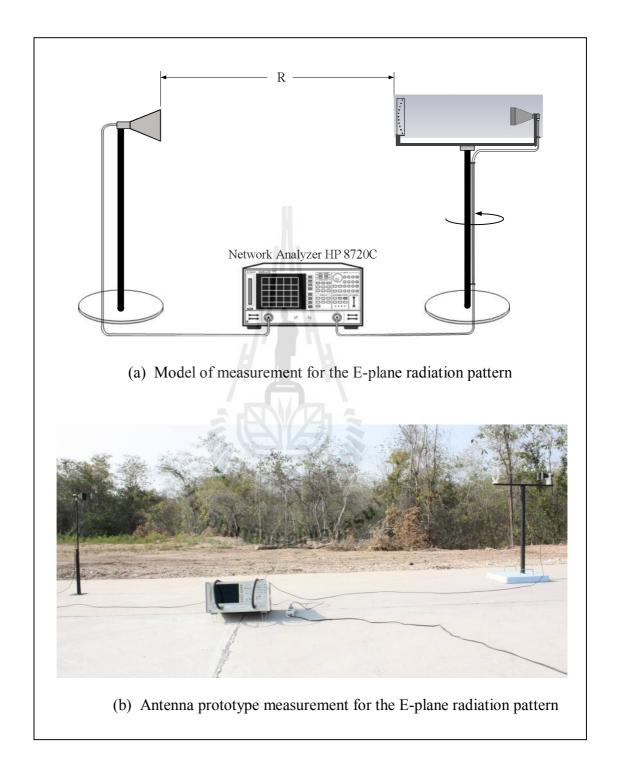
**Figure 5.16** Measurement set up for the radiation pattern of the prototype of Type-D rectangular horn.
