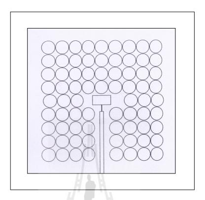
**Figure 2.6** A patch antenna on the PBG substrate formed by four holes in a square lattice (Gonzalo, Maagt, and Sorolla, 1999).
