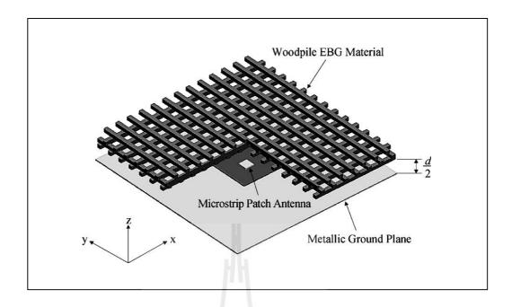
**Figure 2.10** A high gain antenna design using the woodpile EBG structures (Weily *et al.*, 2005).
