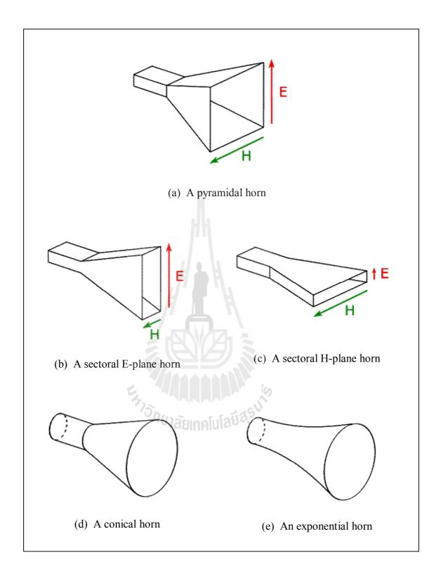
Figure 3.1 Typical horn antenna configurations (http://en.wikipedia.org).
