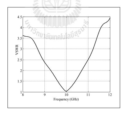
Figure 5.22 Simulated VSWR of a Type-D circular horn with PEC arm.
