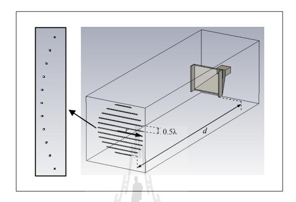
**Figure 4.20** A rectangular horn antenna with two side-wing slabs and the designed woodpile EBG (Type-D rectangular horn).
