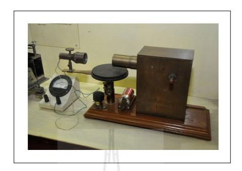
**Figure 2.1** The first horn antenna as the microwave apparatus at the Bose Institute, Kolkata, India (http://en.wikipedia.org).
