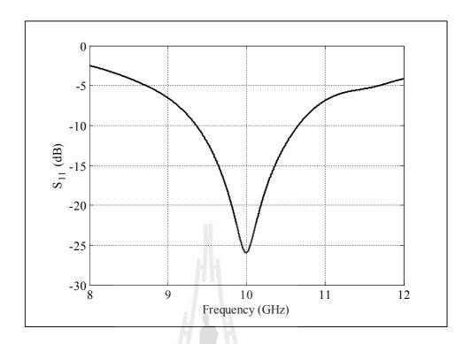
Figure 4.13 Simulated result of reflected power  $(S_{11})$  of a Type-B rectangular horn.
