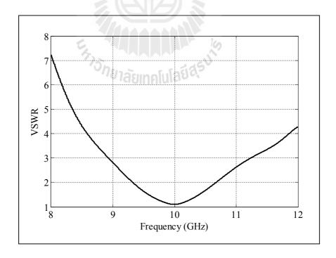
Figure 5.7 Simulated VSWR of a Type-D rectangular horn with PEC arm.
