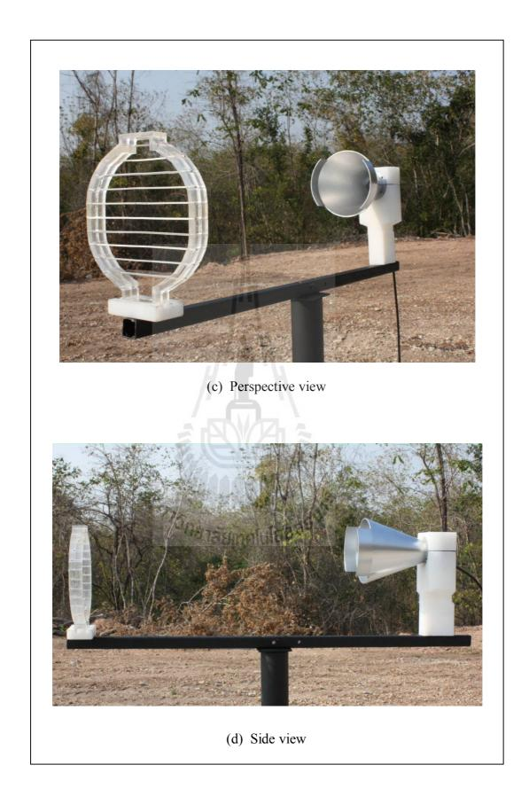
Figure 5.20 The structure and prototype of a Type-D circular horn (Continued).
