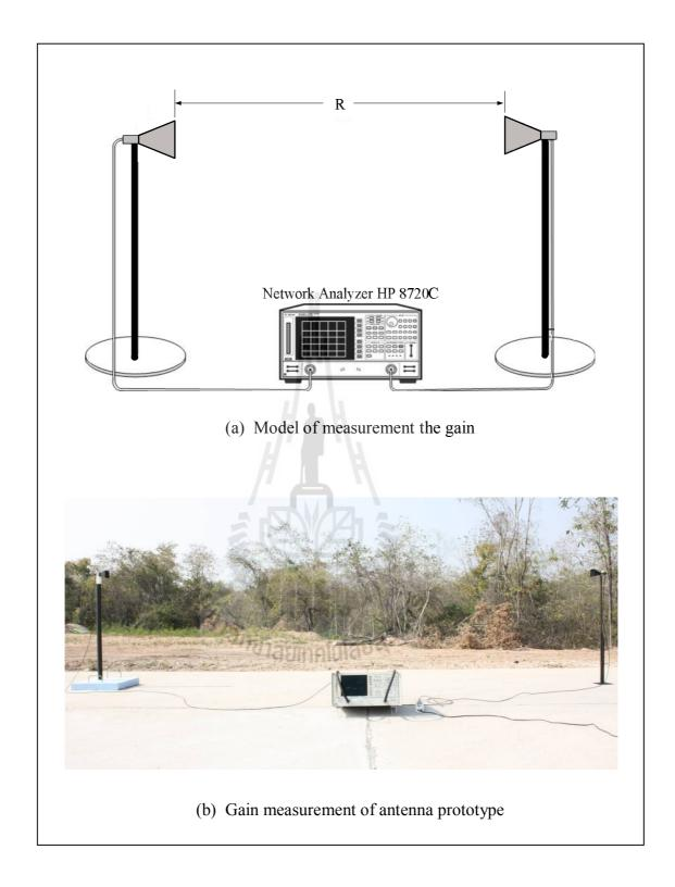
Figure 5.18 Gain measurement of a conventional rectangular horn antenna.
