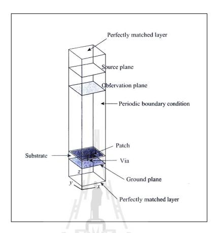
**Figure 3.10** The full wave FDTD model for the EBG analysis (Kim, Yang, and Elsherbeni, 2007).
