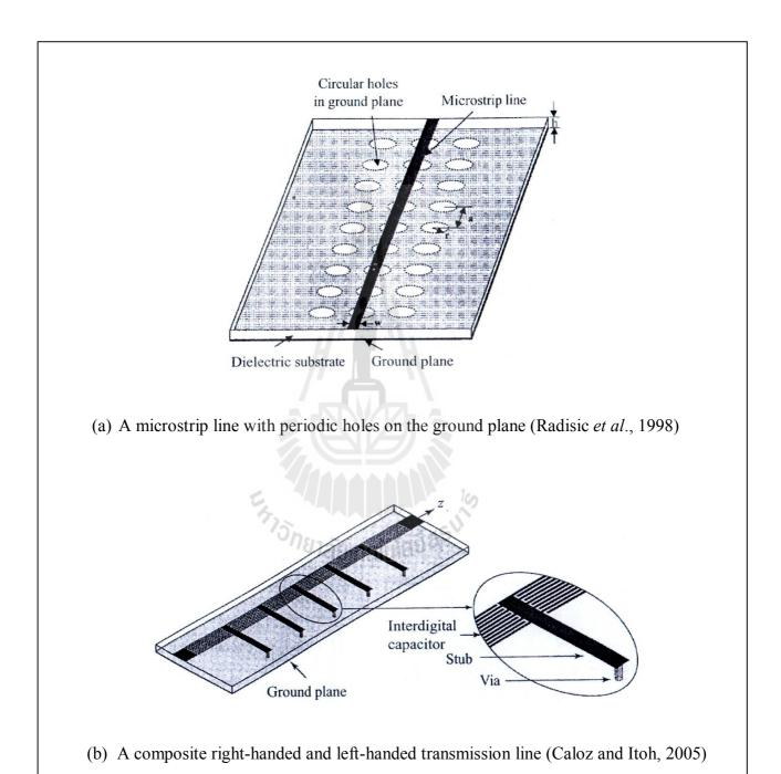
Figure 3.4 The 1D EBG transmission lines.
