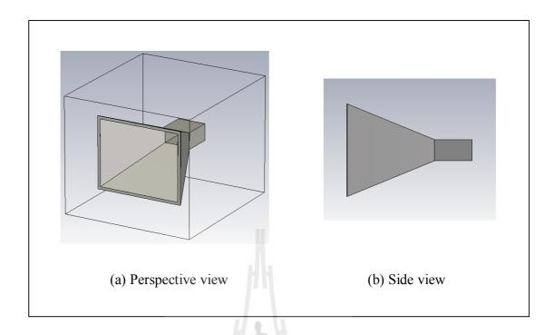
Figure 4.8 A conventional rectangular horn antenna (Type-A rectangular horn).
