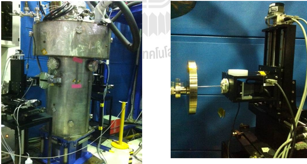
Figure 3.4 The flipping coil setup for measuring first and second field integral of SWLS.
