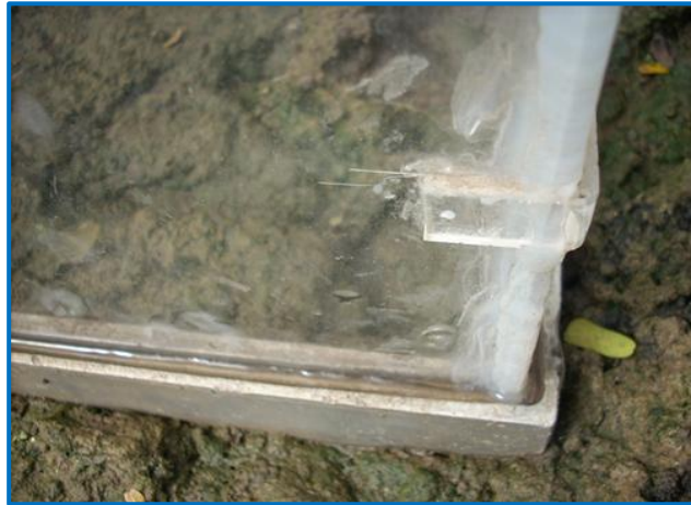
Figure 3.12 Water fill in the groove of the aluminum chamber.
