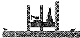
Jackup Rig For drilling in water depths from 15 ft to +/- 350 ft.
