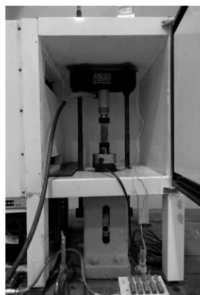
Fig. 2 Salt specimen placed in the consolidation load frame and inside the cooling system for low temperature at 273 K.
