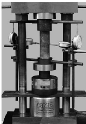
Fig. 1 Salt specimen placed in a compression machine under room temperature (about 303 K).
