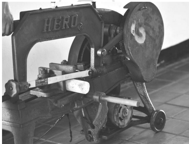
Figure 3.2 Salt core is dry-cut by a cutting device.
