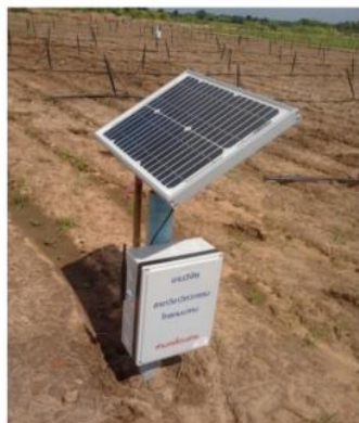
Fig. 10 SSN base station (Coordinator) installation in SUT farm
