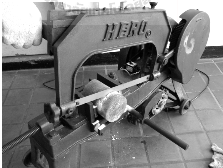
Figure 3.2 Salt core is dry-cut by a cutting saw.
